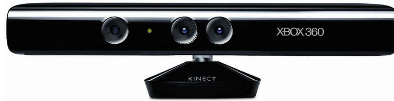
Figure 3.1.: The original version of the Kinect sensor device. Both the RGB and IR cameras are located in the middle, the IR projector can be seen to the left. (Image taken from Microsoft press release)
